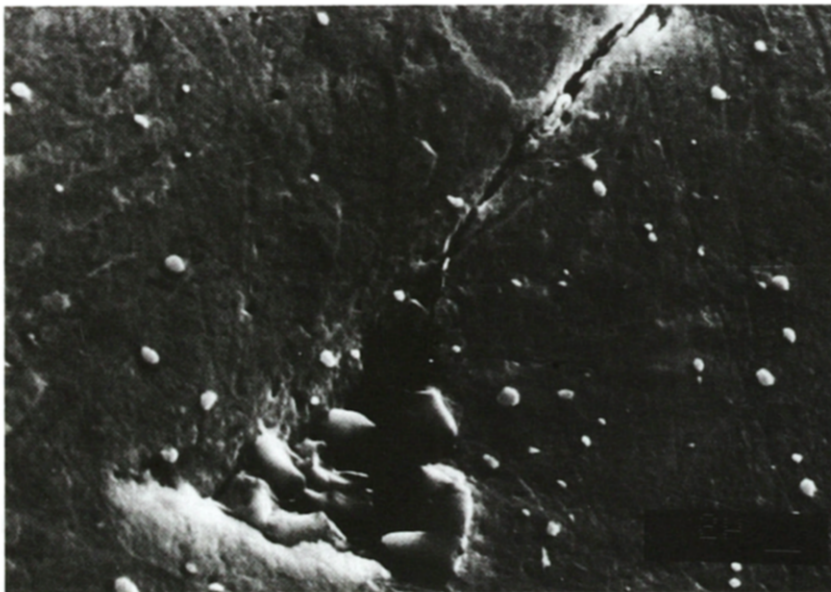
FIG. 4. Structure of steel with 0.1% carbon ( \times 5000 ) at a depth of 5 mm after treatment with titanium powder.
