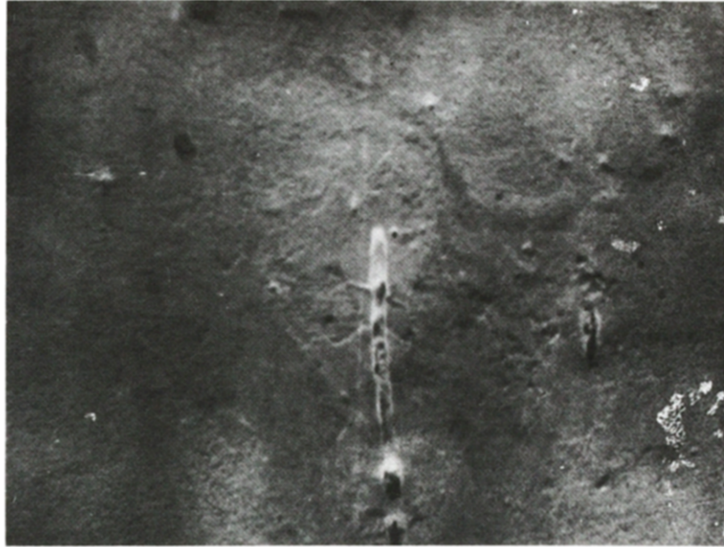
FIG. 5. Structure of steel with 0.45% carbon ( \times 2000 ) at a depth of 7 mm after treatment with copper powder.
